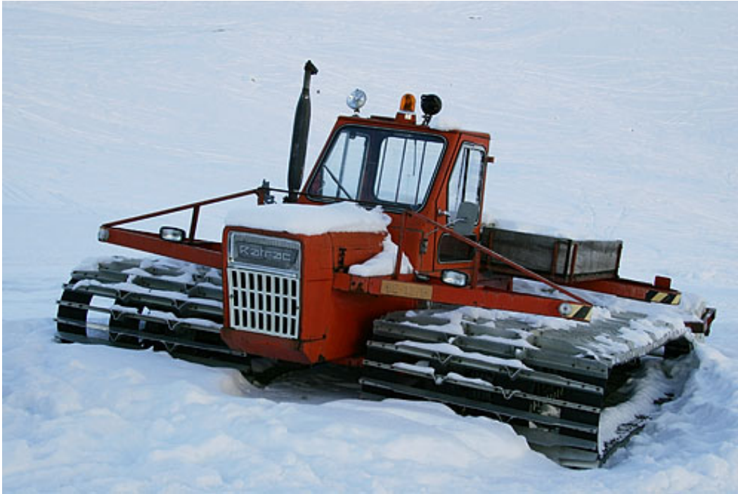
Figure 19. A “ratrak,” which is a snow grooming machine that can be used to harvest biomass in paludiculture with less damage to the soil than conventional harvesters. Photograph by Picswiss.
